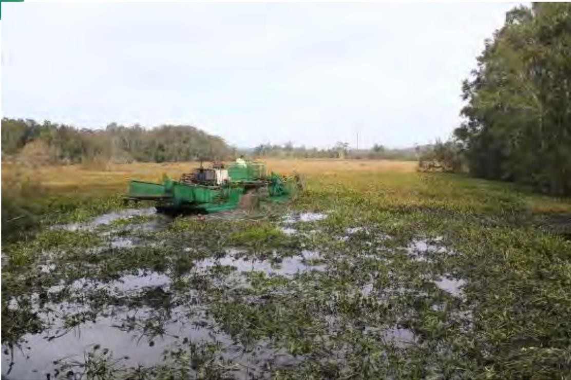
**Figure 23: Tuggerah Lagoon –removal of water hyacinth with the truxor**
